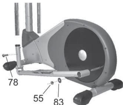
Place the rear end of the left pedal crank on the left rear shaft. Next place the washer and locking nut on the shaft. Tighten the locking nut fingertight. Repeat the procedure on the right side.
