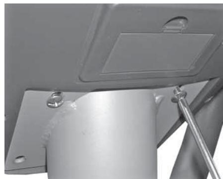
Connect the cables from the front tube and console. Push the connected cables inside the front tube and place the console on top of the front tube. **NOTE!** Beware not to damage the cables! Attach the console with four screws. Remove the protective films from the console display.
