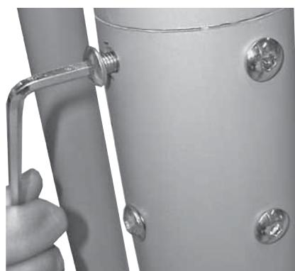
Thread the brake wire and the console cable into the front tube so that both go behind the lateral tube inside front tube. Lead the brake wire out of the opening for the resistance adjustment knob and the console wire from the upper end of the front tube. Push the front tube inside the frame tube: beware not to damage the console cable! Attach the front tube with six screws tight.
